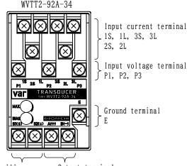
Auxiliary Output terminal supply terminal A(+), B(-) $S1(\pm)$ ,  $S2(\pm)$
