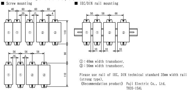
How to install this product in a IEC / DIN rail. The claw of the upside of the slot for rail mounting in the bottom of this product is put in a rail. This product is fixable by pushing in the direction of an arrow below.
