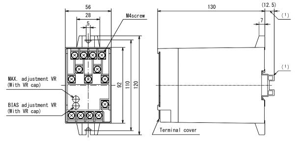
Note(1) Dimensions when IEC/DIN rail (height 15mm) is installed. (Please use a rail with a width of 35mm) The terminal cover is standard equipment.
