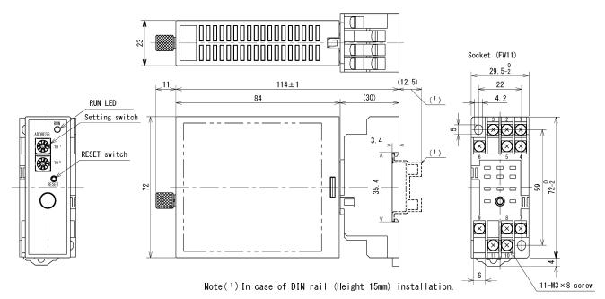
Socket: Standard is M3 $\times$ 8 (dated washer) screw. M3 $\times$ 8 double washer type screw can support by designation, too. In designation of a M3 $\times$ 8 double washer type screw, please designate as socket type FW11-W at the case of an order.
