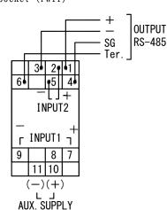
By short-circuiting Ter. and —, a terminating resistor of  $100\,\Omega$  is connected.
